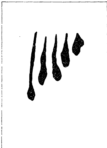
Fig. 29. Viscosity shape of the spot of PS ( M_w = 8.7 \cdot 10^5 ) in TLC on KSK silica gel in Bz. Amounts of PS (left to right): 40, 30, 20 and 10 \mu\text{g} .
